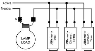
When replacing existing three or more way switching with multi-way dimming/timing/switching using LEDsmart+, the existing strapper wires can be re-used. No new wiring is required.
