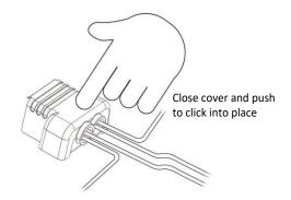
The terminal block can then be cable-tied to the rear of the dimmer housing utilising the two loop holes
