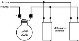
When replacing existing two-way switching with two-way dimming/switching using LEDsmart+, the existing two-way strapper wires can be re-used. No new wiring is required.
