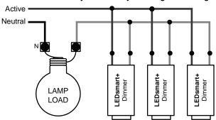
When replacing existing three or more way switching with multi-way dimming/switching using LEDsmart+, the existing strapper wires can be re-used. No new wiring is required.
